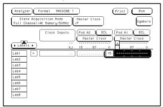
**c** Select Master Clock, then select a double edge for the clock of the pod under test. Turn off the other clocks.
